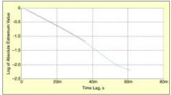
Figure 13. Damping ratio estimation from the decay curve of the correlation function.
