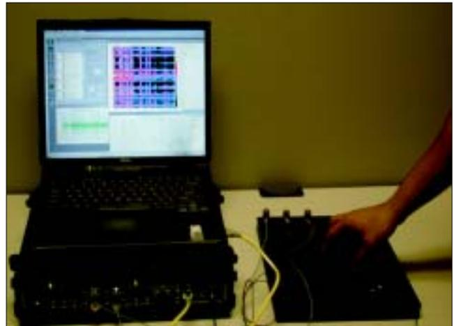
Figure 2. PULSE™ multi-analysis portable system connected to test plate; hand-tapping excitation is demonstrated.
