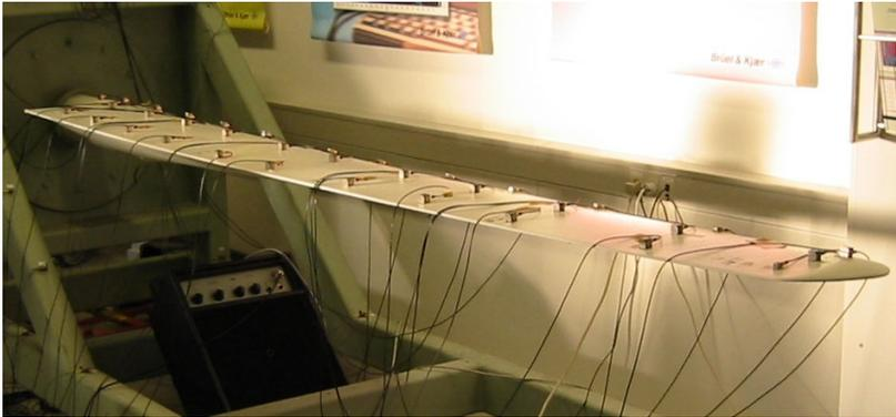
**Figure 2, Test object, 1:5 scale wind turbine wing**
