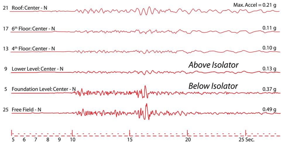
Figure 1: Strong motion records from a 7-story base-isolated hospital in Los Angeles (upper left). Accelerometers are mounted above and below the isolators (upper right). The accelerations recorded in the 1994 Northridge earthquake (lower) clearly show reduction above the isolators relative to the motion at the foundation and in a parking lot nearby.
