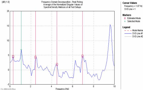
**Figure 6.** Dominant frequencies and viscous damping coefficients
