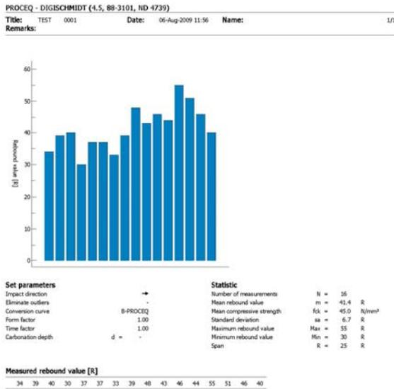
Figure 3. Graphic output for the strength at a given point
