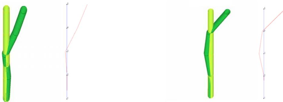
**Figure 7.** Vibration shape at  $f = 0.29$  Hz and  $f = 1.07$  - experimental
