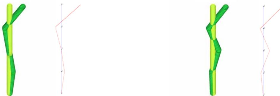
**Figure 8.** Vibration shape at  $f = 2.44$  Hz and  $f = 4.49$  Hz - experimental
