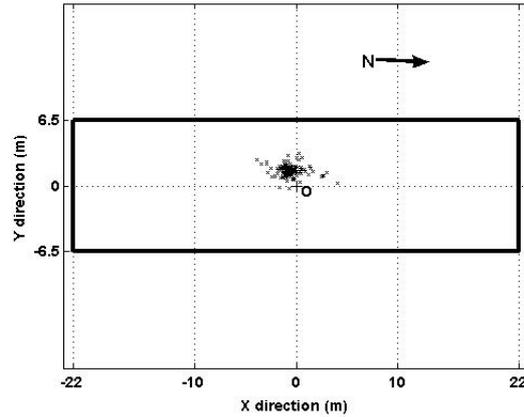
**Figure 5: Spatial distribution of the rotation centres of the building for the 178 recordings**
